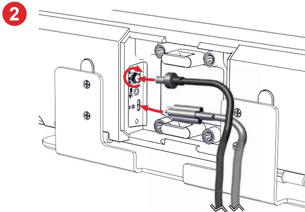
3. Attach other cables (Audio I/O, Ethernet) as necessary and route all cables through the strain relief stubs. The covers rotate up or down to contain the cables.
